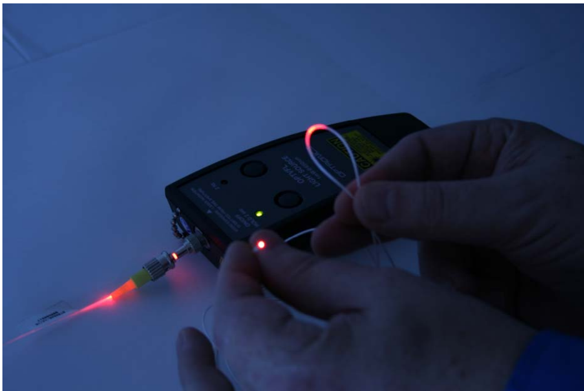
Picture 1: Detecting Macrobending with a VFL
